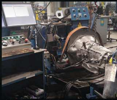
All units are 100% dynamometer tested.
