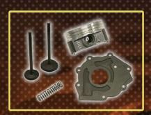
JASPER upgrades 4.6/5.4/6.8 engines with nitrided valves, JASPER designed pistons, and (on 3-valve VVT V8 engines) a high-volume oil pump with a higher pressure relief valve spring and updated backing plate to improve durability and operation.
