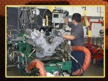
JASPER engines undergo live-run testing using state-of-the-art data acquisition to check compression, vacuum, and oil pressure to ensure reliability.
