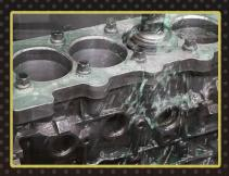
For the best possible cylinder wall geometry, JASPER utilizes torque plate honing with a torque plate and specially-designed ARP2000° head bolts.
